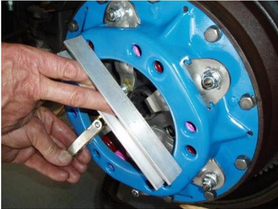
The clutch measurement for the 6 fingers is from where the throw out bearing contacts the fingers to a straight edge laid across the face of the pressure plate.
